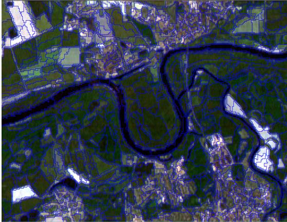
**Figure 3:** Segmentation result as provided by eCognition for scale parameter 10.
